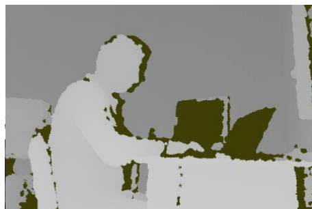
Figure 5. Depth image provided by Kinect sensor
