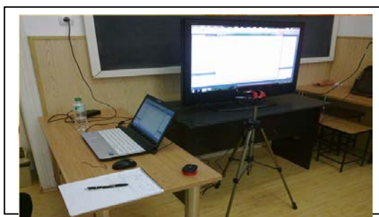
Figure 7. Kinect sensor system for postural deviation analysis
