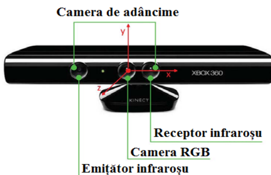
Figure 2. Kinect sensor parts
